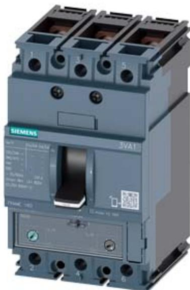
CIRCUIT BREAKER 3VA1 IEC FRAME 160 BREAKING CAPACITY CLASS N ICU=25KA @ 415 V 3-POLE, LINE PROTECTION TM240, ATAM, IN=16A OVERLOAD PROTECTION IR=11,2A ...16A SHORT CIRCUIT PROTECTION II=10...20 X IN BUSBAR CONNECTION UNDERVOLTAGE RELEASE (UVR) 120-127 V AC 50/60 HZ
